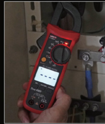
NCV multi-segment display and audio/visual alarm
