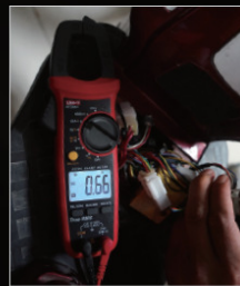
Small range measurement, accuracy guarantee range 1%-100%
